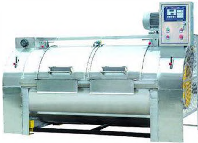
200Kg-400Kg全不锈钢变频调速洗染机 200kg-400kg Full-Stainless Steel Frequency Conversion Speed Regulating And Dyeing Machine
